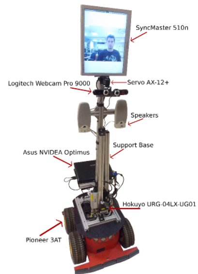
Fig. 1. DOKBot, a semi-autonomous avatar for telepresence applications.
