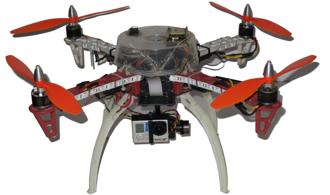
Fig. 5: Custom Built UAV. It is based on the DJI F450 frame and uses an ArduPilot Mega 2.6 as flight controller. In this picture the UAV's camera has been upgraded to a GoPro Hero 3+ Black Edition, but at the time the experiments were performed the vehicle was equipped with a Mobius ActionCam Lens B, which is comparable to the GoPro Hero 3 White Edition. It also uses a brushless motor gimbal to stabilize the image.
