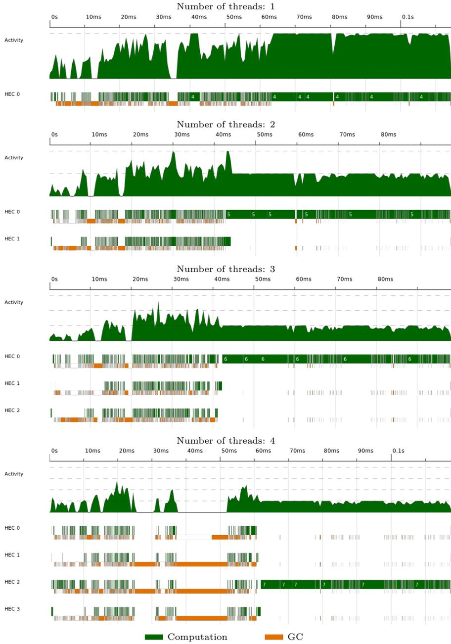
Figure 4: Profiling information for the Factorial benchmark. Notice how the second half of the execution is a uniquely sequential process, in this case, dedicated to writing the large output.
