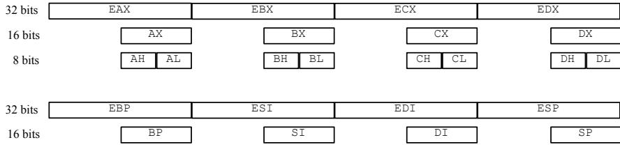
**Figure 1. General purpose registers of the x86 architecture**
