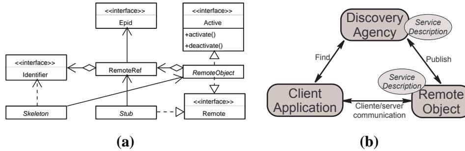
Figure 4: (a) Remote object representation. (b) Service-oriented architecture.
