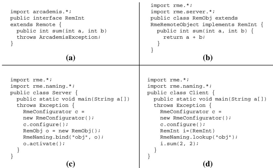
**Figure 7: (a)Remote Interface. (b)Remote Object. (c)Server. (d)Client.**
