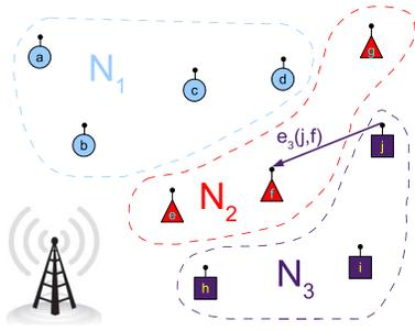
Fig. 1. A scenario where different WSNs are deployed in the same location. We see three networks,  $N_1$ ,  $N_2$  and  $N_3$ , and a possible cooperation edge  $e_3(j, f)$ , where node  $f$  accepts data of network  $N_3$  coming from sensor node  $j$ .
