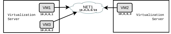
Fig. 7: Topology used to evaluate flow configuration time, packet forwarding latency, and broadcast latency.
