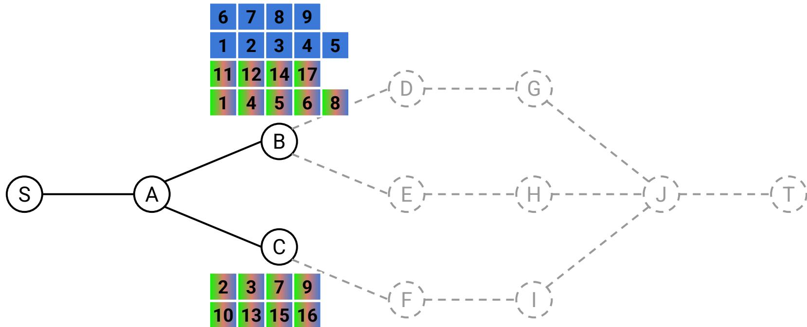
All packets traverse the link A-B, MCA infers that A's hash function does not consider ports
