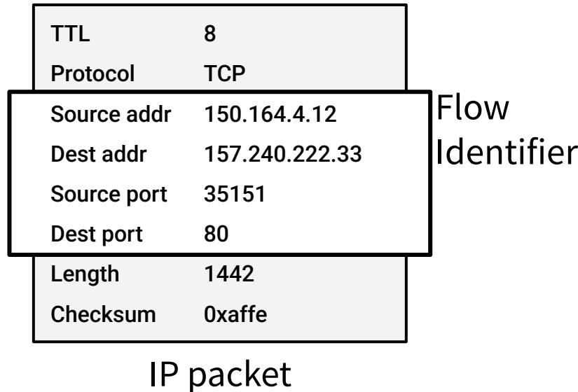
The load balancer extracts a set of bits called the **flow identifier** from the packet
