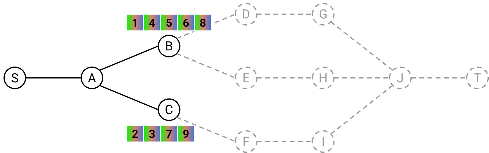
MCA sends 9 probes with TTL = 2, detects load balancing, and sends additional probes to check for more links
