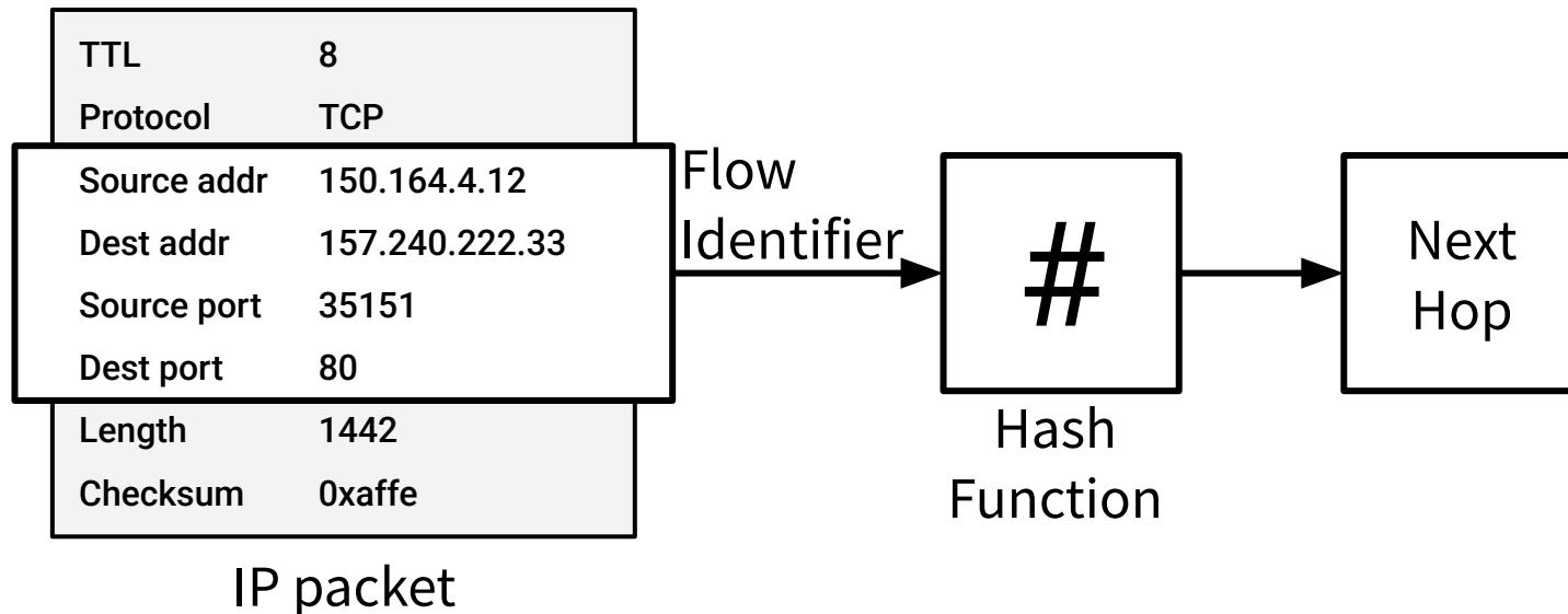
MCA allows varying most bits in the IP, TCP, UDP, and ICMP headers
