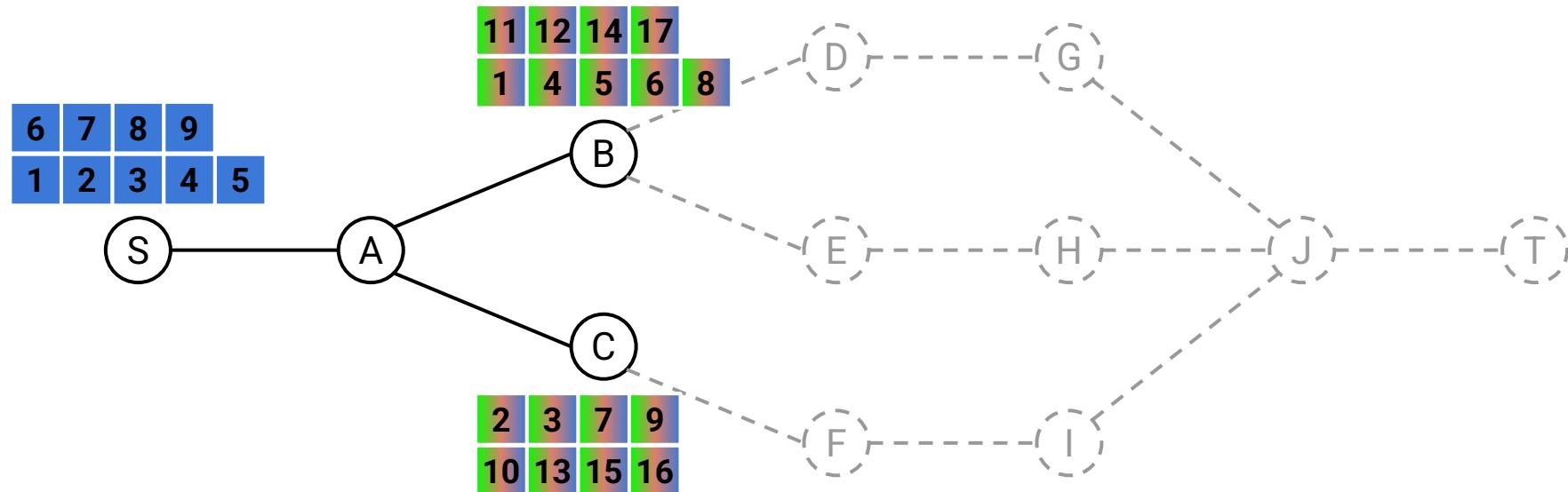
MCA sends 9 probes varying a subset of bits in the packet header, like the port numbers
