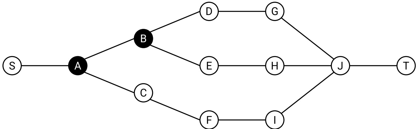
Routers A and B perform load balancing
