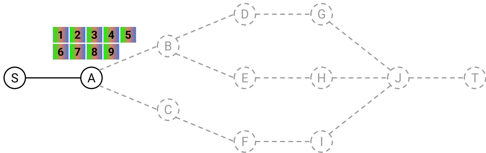
MCA sends 9 probes with TTL = 1 varying all bits, does not find any load balancing, and proceeds to the next hop
