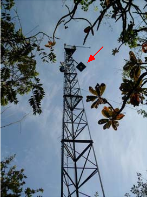
Fig. 1. The cerrado-savanna phenology tower (18m tall), where the digital hemispherical lens camera was set up (red arrow) attached in an iron arm facing northeast.
