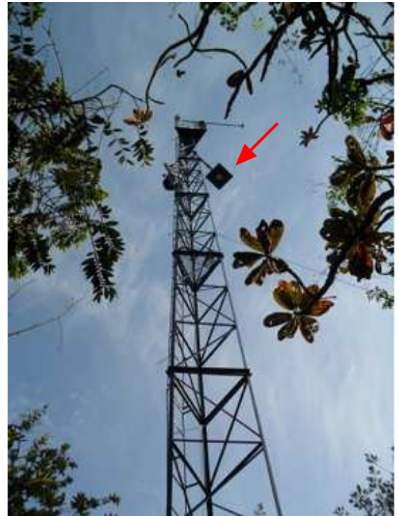
Figure 1: The cerrado-savanna phenology tower (18m tall) at Itirapina, São Paulo, Southeastern Brazil, where the digital hemispherical lens camera was set up (red arrow) attached in an iron arm facing northeast.
