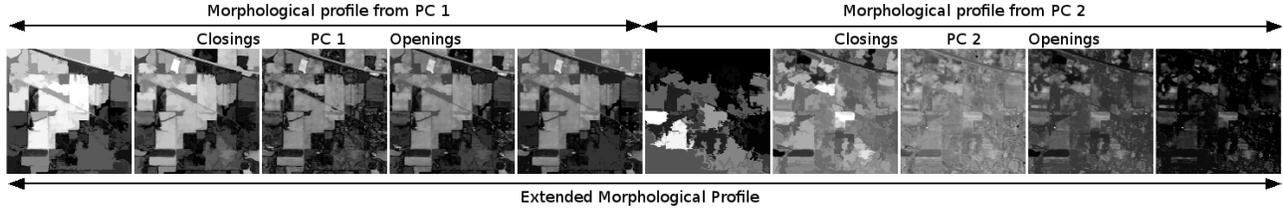
**Fig. 1.** Example of the EMP on the Indian Pines data set. Number of PCs = 2, discrete disk SE of radius and increasing step equal to 4, and number of openings/closings equal to 2. Total of 10 features in the EMP scheme.
