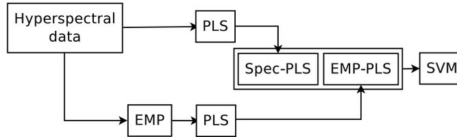
**Fig. 2.** Diagram of the SpecEmpPLS-SVM approach. The PLS is used to encode both spectral and spatial information which is interpreted by the SVM classifier later.
