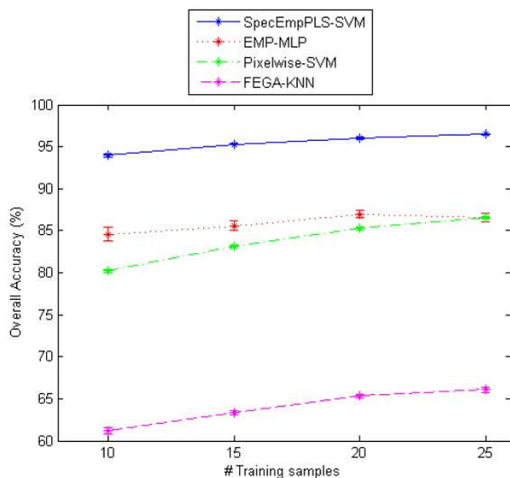
**Fig. 4.** Results for the *Indian Pines* data set as a function of the samples used for training (in percentage). The star symbols (\*) are the averages of 30 runs and the vertical bars are the respective CI.
